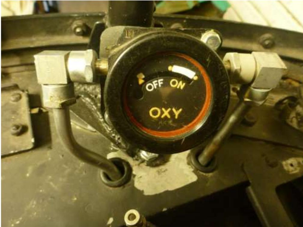
The left hand pipe comes up through the turret floor from the (missing) Rotating Services Joint whilst the right hand pipe heads down to the Economiser. There were no fixtures or fittings in the Economiser position which is near the floor by the gunner's left foot. The mountings were produced following inspection of similar installations and reference to the turret manuals. Once done they were riveted to the turret skirt.
