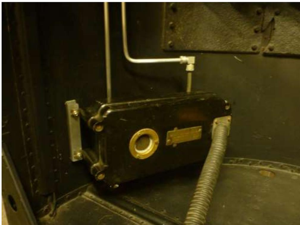
Next comes the protective cover – not a bad idea given the position of the Economiser. This is a large alloy box that I made using the schematic drawing in the manual – the box is then bolted to the turret skirt.
