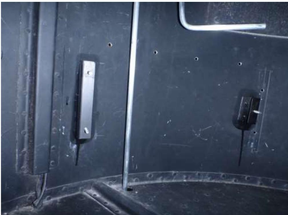
The Economiser is then simple to bolt in and the right hand pipe can be connected. The 90 degree alloy adaptor seen here is borrowed from the oxygen indicator to get the correct fit. The turret actually needs three of these adaptors if anyone has any. The flexible oxygen hose then runs off up to the gunner.
