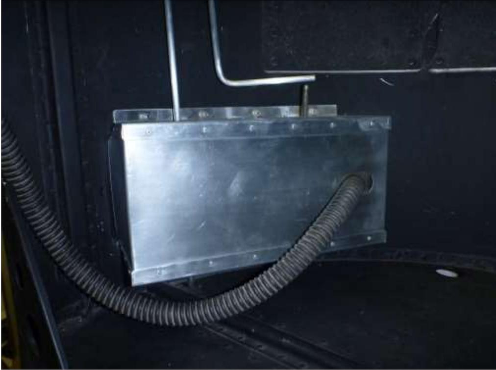
Finally for the oxygen system, a clip was fitted to the original position by the gunner's left elbow to store the oxygen connector. Again, this hose and connector are borrowed from the FN-5, so another example will need to be found.
